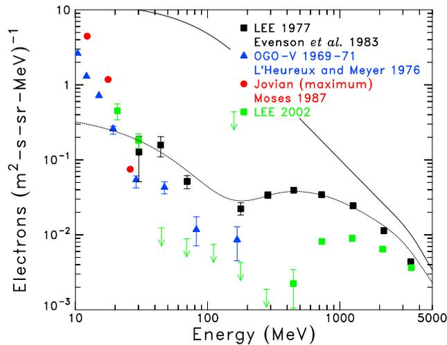
**Figure 4.** Measurements of the cosmic electron spectrum. Data for 1977, estimated local interstellar spectrum (solid line), and fit to the data are from *Evenson et al.* [1983]. Also shown are a spectrum for 1969–1971 from *L'Heureux and Meyer* [1976] and a 1 AU Jovian electron spectrum [*Moses*, 1987].
