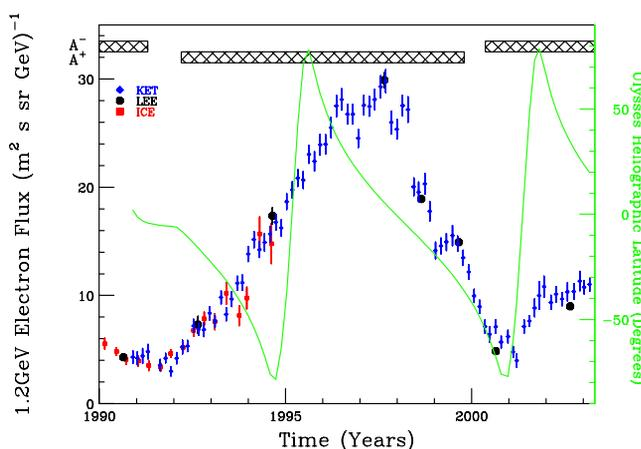
**Figure 5.** Measurements of electrons as a function of time at a rigidity of approximately 1.2 GV. The large solid circles are data from the LEE series of balloon flights. The red squares are data from the ISEE-3/ICE spacecraft and the blue diamonds are data from KET/Ulysses. The green line shows the heliograph latitudinal location of the Ulysses spacecraft. Epochs of well-defined heliospheric magnetic polarity are indicated by shaded rectangles.
