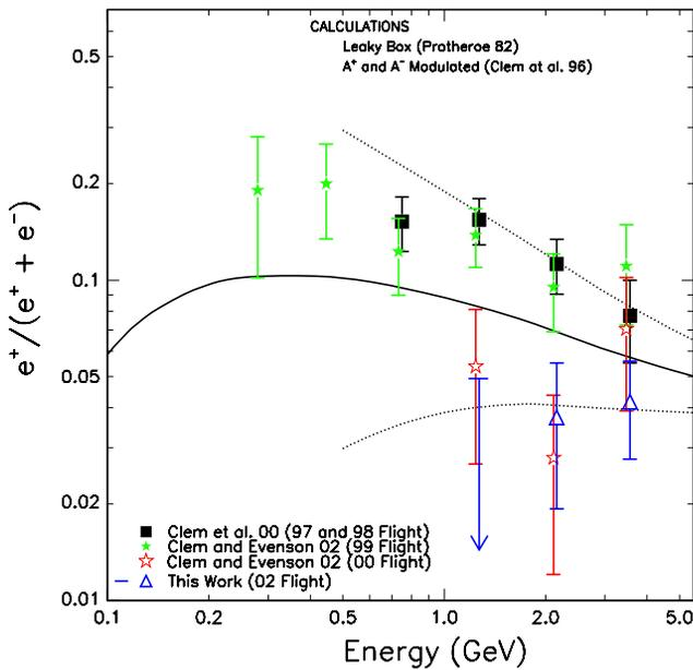
**Figure 1.** Compiled AESOP balloon instrument measurements and calculations of the positron abundance as a function of energy for different epochs of solar magnetic polarity. Solid line is the local interstellar space abundance as calculated by *Protheroe* [1982]. Dashed lines are from *Clem et al.* [1996] for A+ (top line) and A-. Solid symbols show data taken in the A+ state, while the open symbols represent data taken in the A- state.
